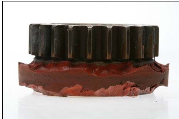
Photo 1. Gear damage to rubber material
