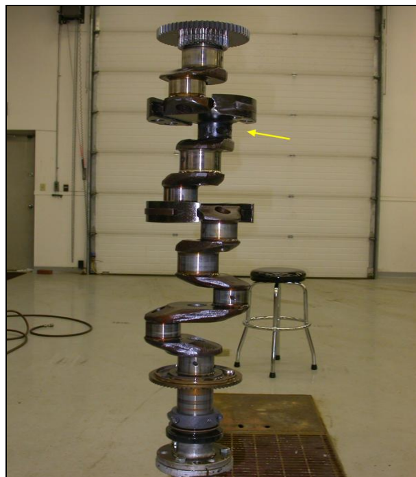
Photo 3. Crankshaft showing heated area
