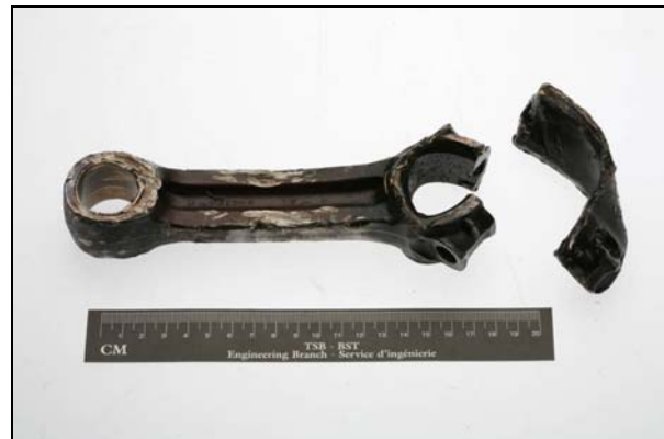
Photo 2. Heat and contact damage to connecting rod 2
