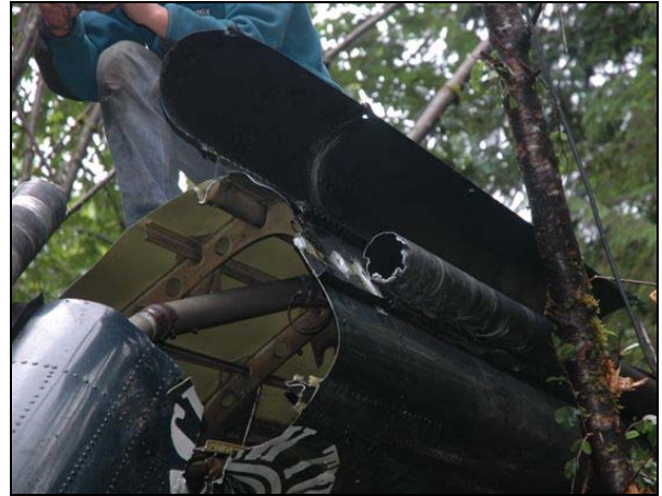
Photo 2. Fractured tail rotor driveshaft
