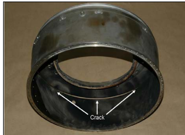
Photo 2. CCH crack detail (N205HQ)
