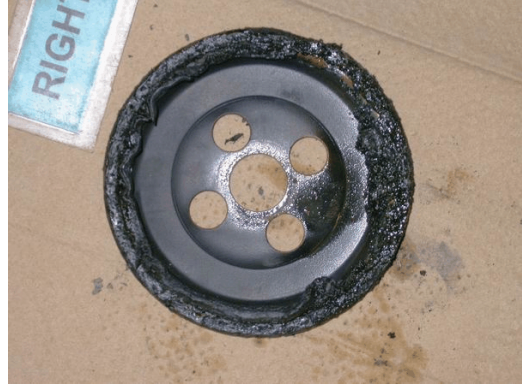
Photo 1. Right-engine converter plate gasket
