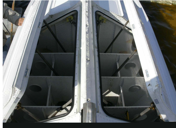
Figure 4 - Bomb doors open (float upside down)
