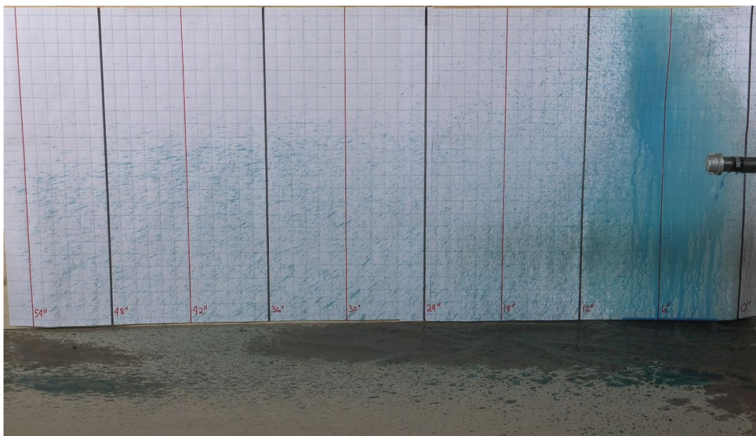
Figure B2. Fuel spray test results in 2 dimensions. Note that the spray would be in 3 dimensions, and that spray near an engine may reflect or drip onto nearby surfaces. (Source: TSB)
