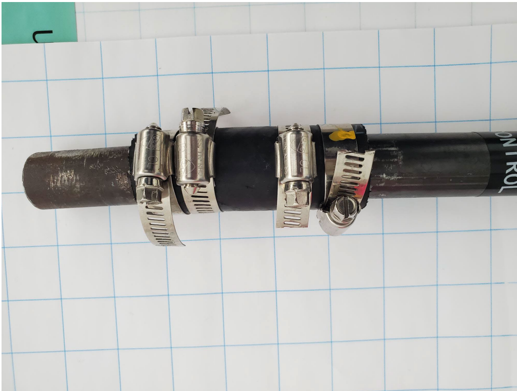
Figure 12. A reconstruction of the final temporary repair (Source: TSB)
