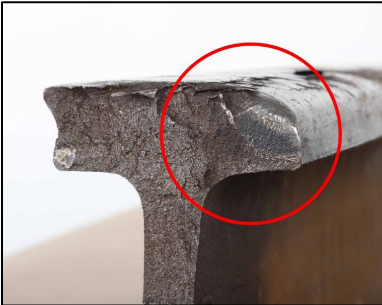
Figure 7. Detail fracture on Rail #1 (Source: TSB)
