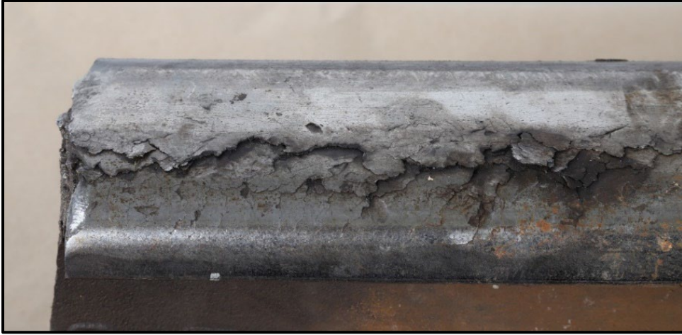
Figure 7. Detail fracture on Rail #1 (Source: TSB)
