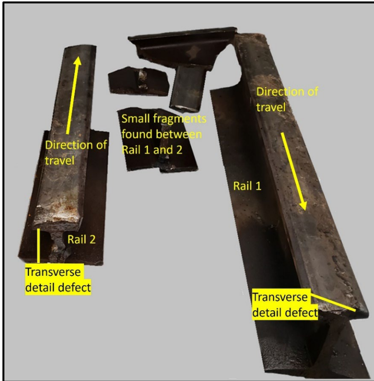
Figure 5. Rail pieces recovered from the occurrence site (Source: TSB)
