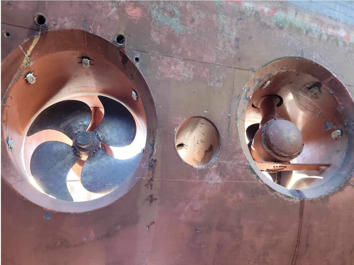
Figure 2. View of the Atlantic Vision 's bow thrusters from starboard (Source: TSB)
