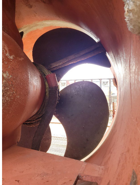
Figure 10. Mooring line wound around bow thruster (Source: Groupe Océan)
