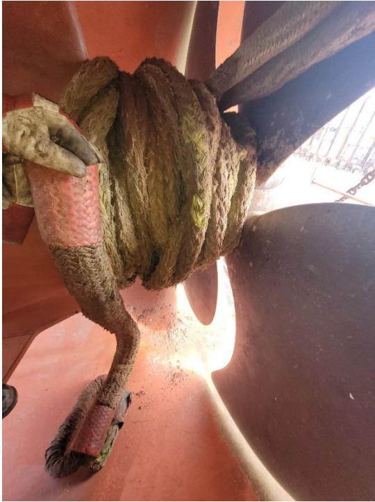
Figure 9. Close-up of mooring line wound around bow thruster (Source: Groupe Océan)
