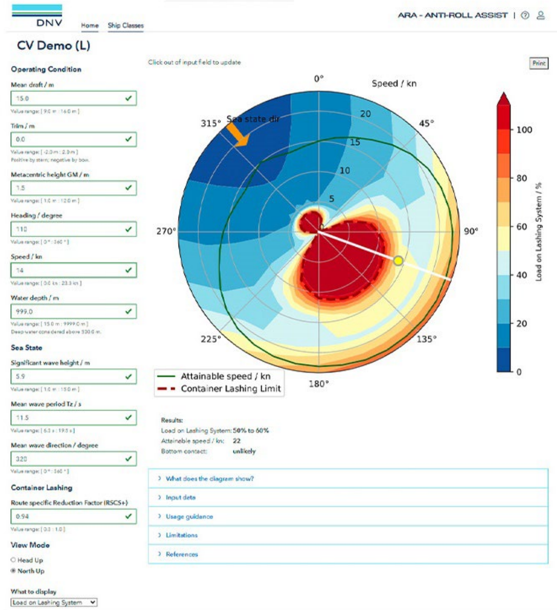
Figure 21. Example of a polar diagram provided by the Anti-Roll Assist app. The red area indicates where the vessel's container lashing limits would be exceeded (Source: Det Norske Veritas, "New DNV anti-roll app helps avoid container loss," (31 May 2022), at https://www.dnv.com/expert-story/maritime-impact/New-DNV-anti-roll-app-helps-avoid-container-loss.html [last accessed 16 July 2024])
