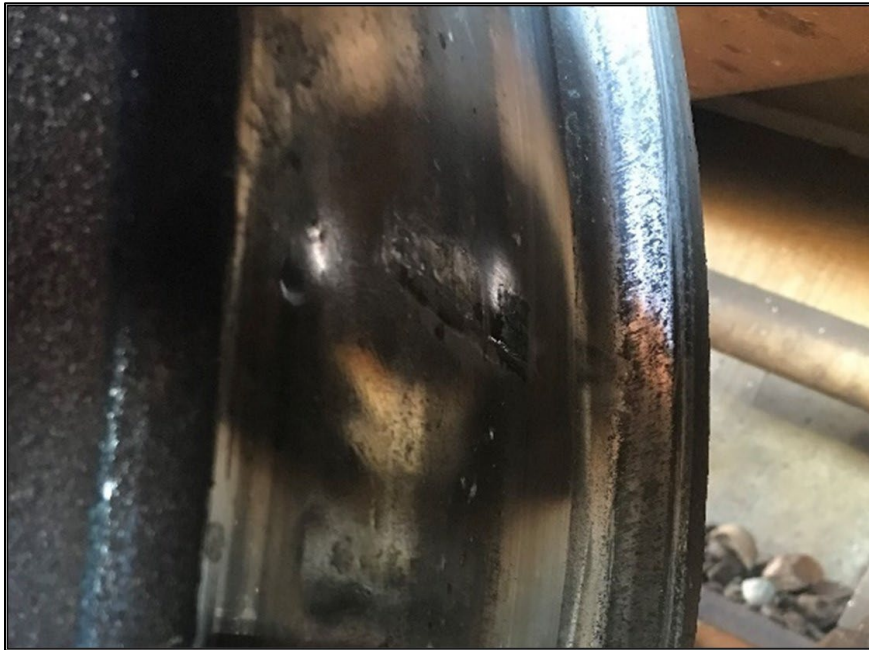
Figure 5. Car CITX 151689 R1 wheel tread impact damage (Source: CP)
