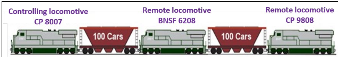
Figure 1. Illustration of the occurrence train's distributed power configuration (Source: TSB)
