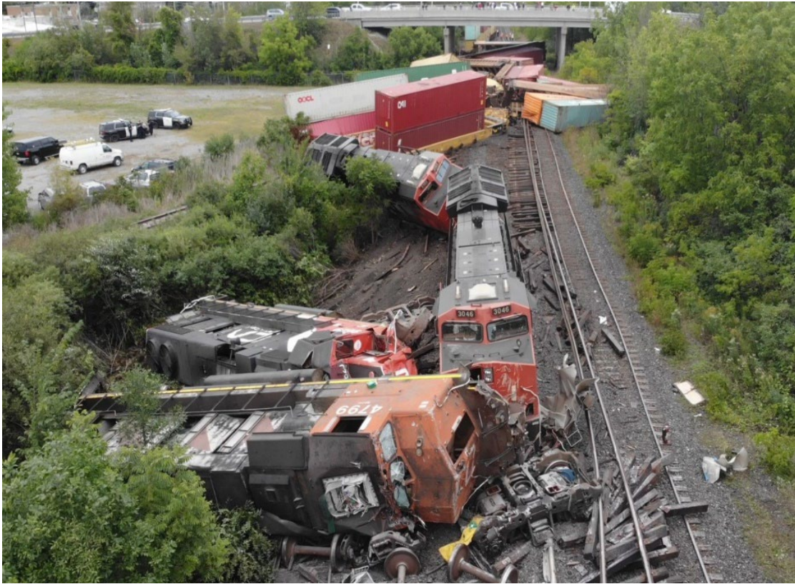
Figure 4. Derailed rolling stock and damaged track after the collision (Source: Ontario Provincial Police)
