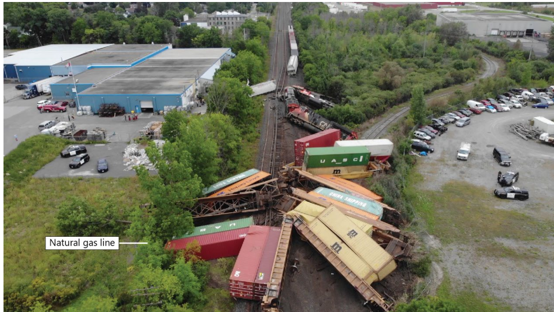
Figure 5. Derailed intermodal car and container near a natural gas line (Source: Ontario Provincial Police, with TSB annotations)
