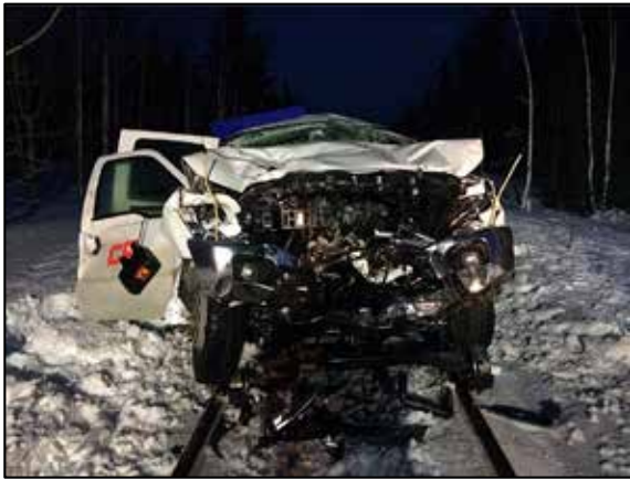
Figure 2. Front view of hi-rail vehicle after collision
