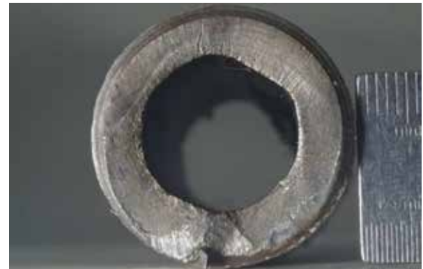
Figure 4. Fracture surface of the threaded portion of the nipple (Source: Trans Mountain)
