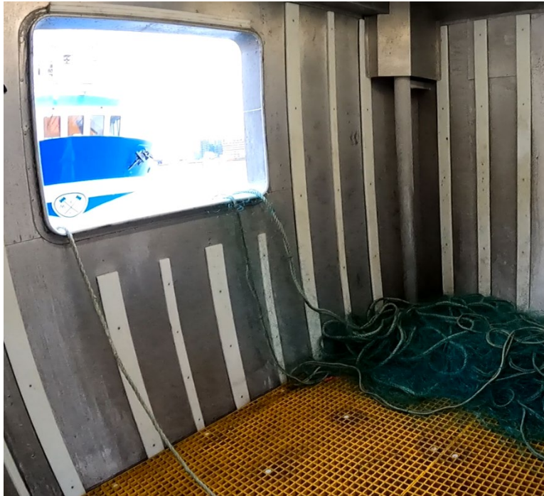
Figure 5. Window in aft bulkhead of the top net house (Source: TSB)
