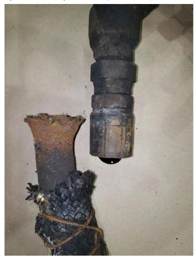
Figure 17. Fuel line aligned to show separation at crimp (Source: TSB)
