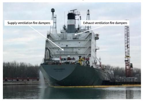
Figure 5. Stern view of vessel's superstructure, showing location of engine room ventilation fire dampers (Source: T&T Marine Salvage Inc., with TSB annotations)
