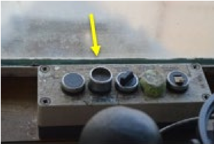
Figure 8. Abort mechanism at the wheelhouse conning station, with the abort button indicated by a yellow arrow (Source: TSB)
