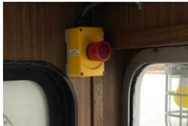
Figure 11. Newly added standardized button for abort mechanism (Source: Ledcor Resources and Transportation Inc.)
