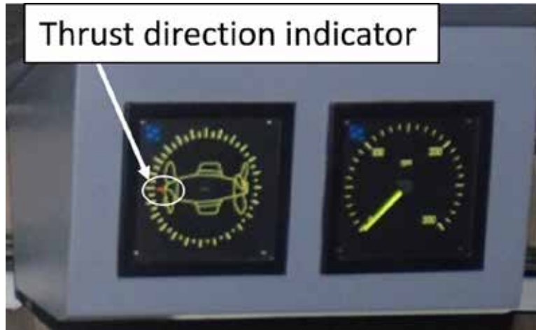
Figure 9. Thrust direction indicator (left) and rpm indicator (right). The red triangle-shaped pointer is circled.
