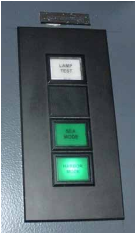
Figure 5. Harbour/sea mode changeover function
