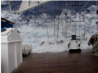
Photo 4. Port deck edge immersed at 29°
