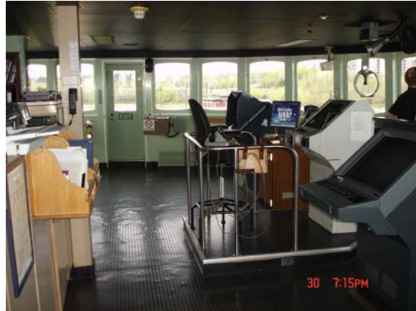
Photo 2. Steering station No. 1, with an ECS display to the left
