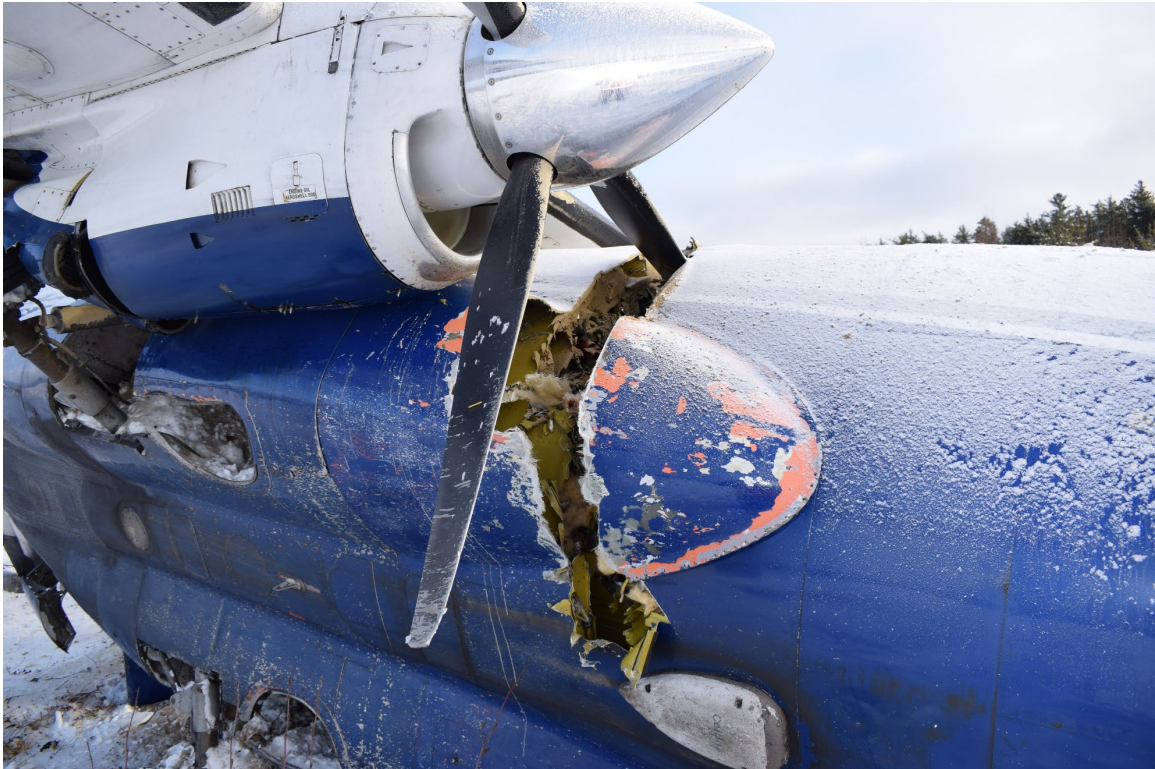
Figure 2. Damage to the fuselage (Source: TSB)
