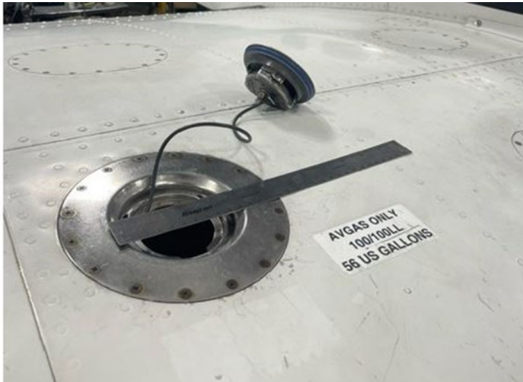
Figure 4. Fuel placard by the right-wing inboard tank filler opening on the occurrence aircraft (Source: SkyCare Air Ambulance)
