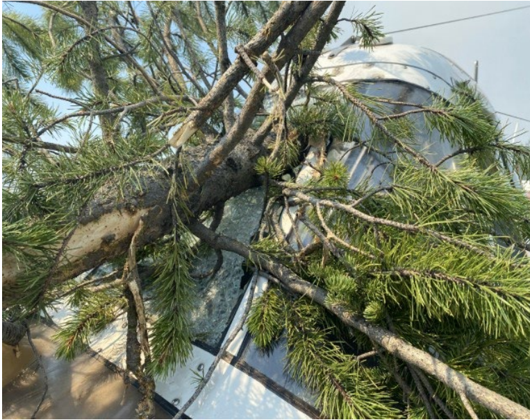
Figure 4. Tree protruding through the front windscreen and into the cockpit of the occurrence aircraft after its collision (Source: Conair Group Inc.)
