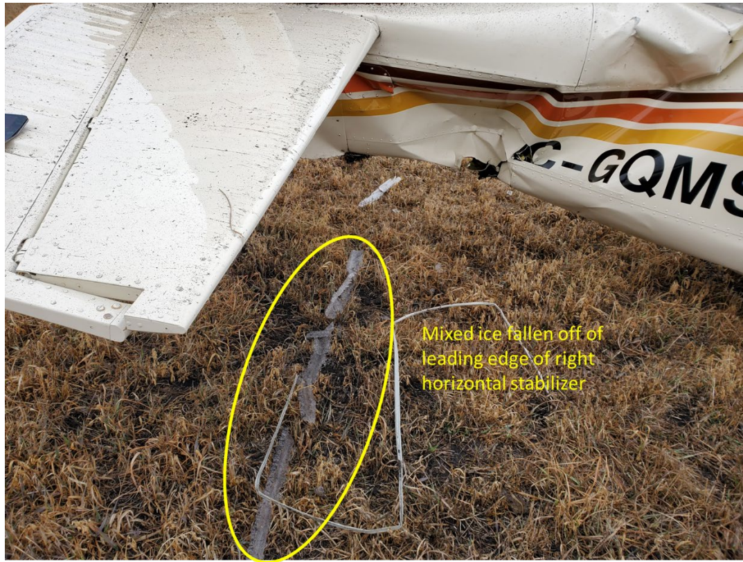
Figure 4. Horizontal stabilizer mixed ice (Source: Royal Canadian Mounted Police, with TSB annotations)
