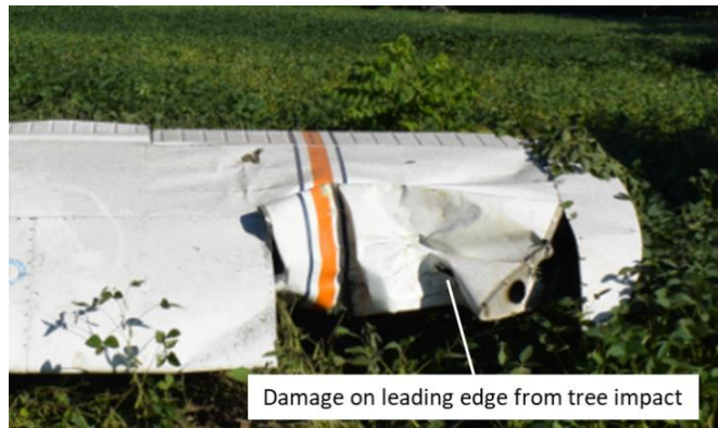
Figure 2. Photo of the damage to the left wing (Source: TSB)
