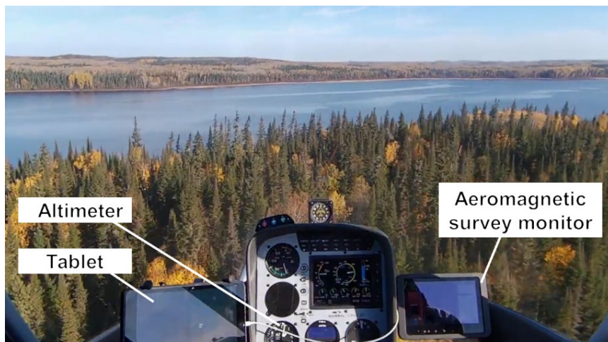
Figure 3. View from the cockpit (Source: Still image taken from a video recorded by the occurrence pilot, with TSB annotations)
