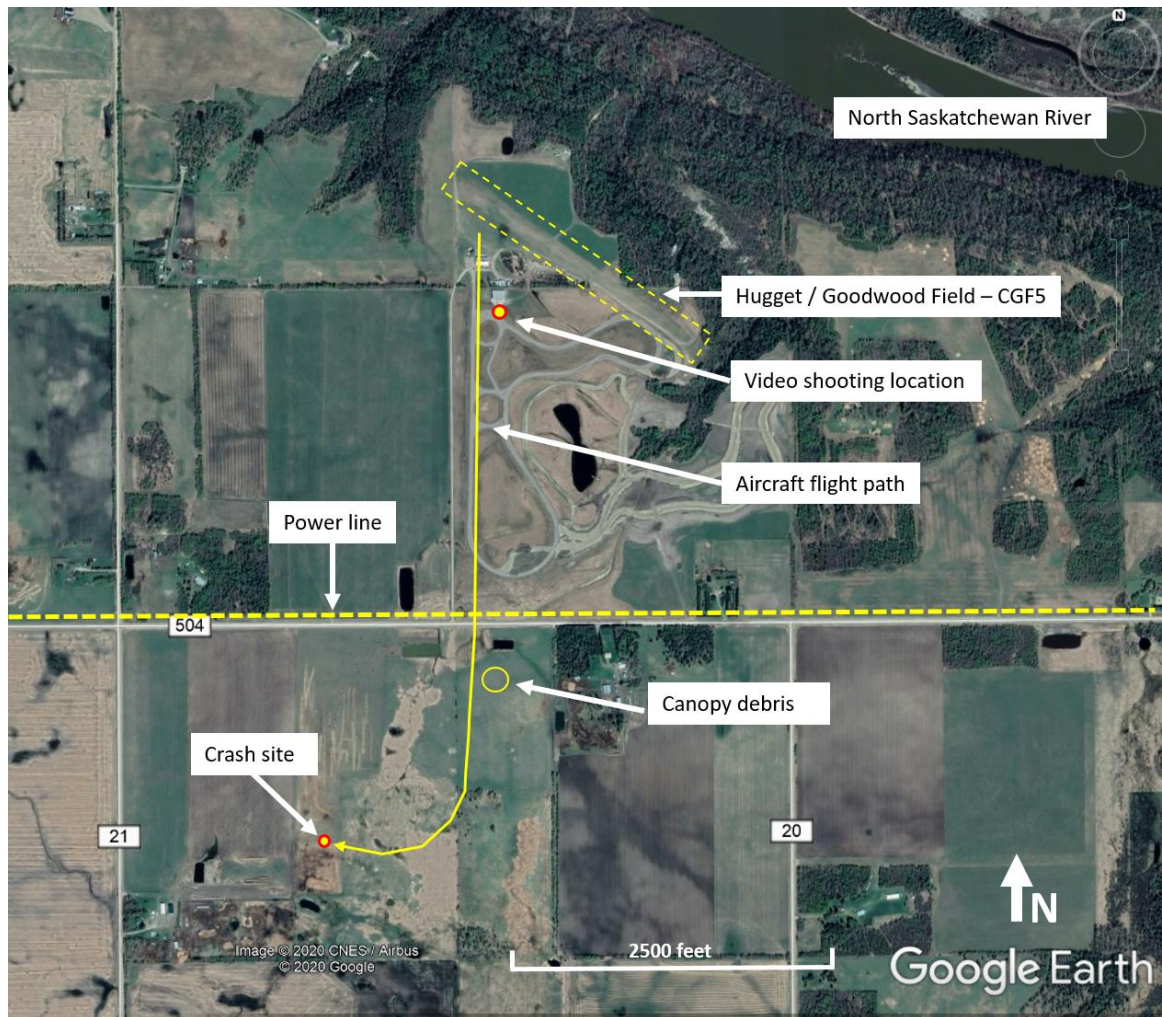
Figure 1. Map showing the occurrence aircraft's flight path, the power line and the accident site (Source: Google Earth, with TSB annotations)
