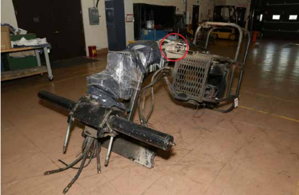
Figure 10. Crane assembly with circle identifying a broken piece of the basket frame
