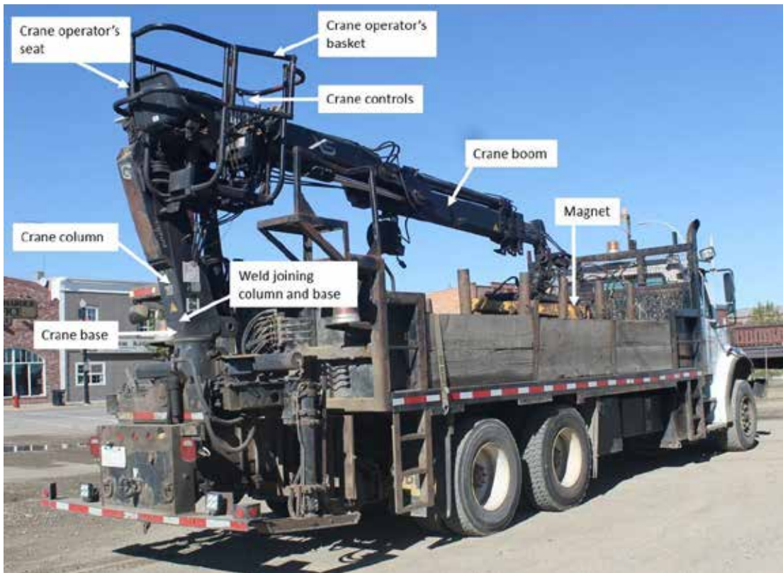
Figure 2. Truck and crane similar to the occurrence truck and crane used by Canadian Pacific Railway Engineering Services
