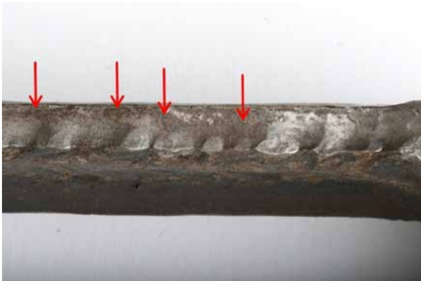
Figure 7. Oxidized fracture surface, indicated by the red arrows
